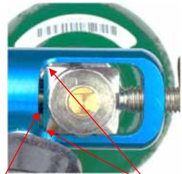
Incomplete washer seal Valve corners interfere with regulator yoke, hindering proper fit
