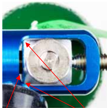
Incomplete washer seal Valve corners interfere with regulator yoke, hindering proper fit
