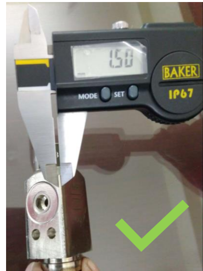
Valve body with 1.50 mm chamfer
