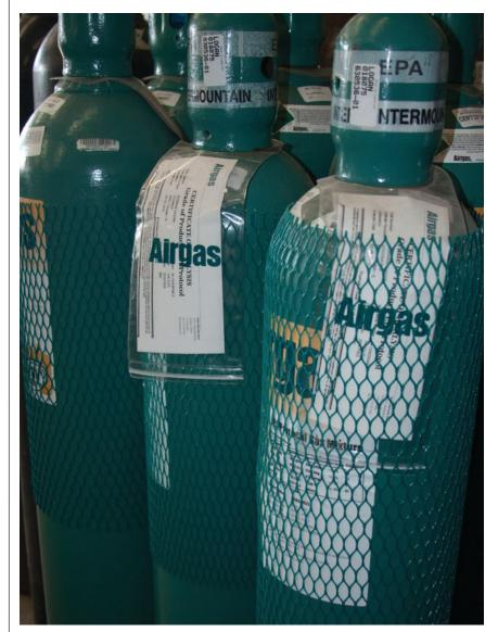
Each cylinder of protocol gas mixture must come with an analytical certification.
